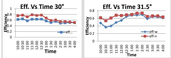
Fig 7: Variation of efficiency with time for 30° tilt angleFig 8: Variation of efficiency with time for 31.5° tilt angle
