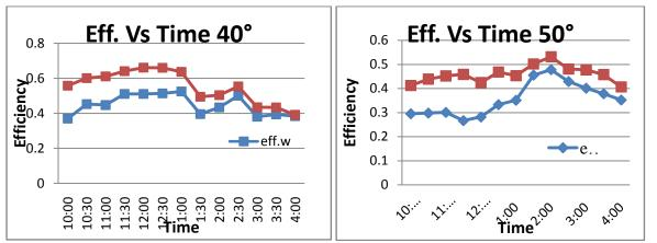
Fig11:Variation of efficiency with time for 40° tilt angleFig 12: Variation of efficiency with time for 50° tilt angle
